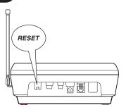
The *RESET* button can be used if an AC power line disturbance causes the answering system to malfunction and become inoperative. Pressing *RESET* does NOT erase any data stored in your system memory.
